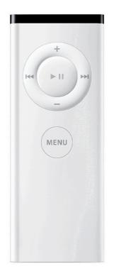
The sphere is controlled by an Apple IR remote (A1176). The remote is simple and the button layout is described under. The remote takes a CR2032 3V battery.
