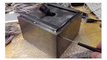
Lift the top part of the housing. Note that two sides of the box are attached to the back of the box and could grip electronic components in the move, pay attention to any restriction to avoid pulling connections out.
