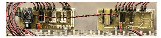
This part could be different in size and layout, based on the iteration on the board design. A custom made board that receives the IR signal from an Apple IR remote control (sensor attached on the 3 pins connector) and drives the motherboards with a signal to either stop, play, reduce or increase the volume (via a distribution board system and the 4 pins connectors). It also acts as a power distribution bay for the power connectors feeding the motherboards (2 pins connectors).
